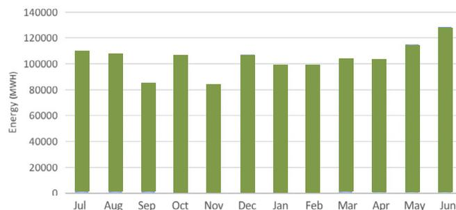
The energy imports over the ZLI totalled 1,223,602.298 MWh during the year. This is equivalent to transmitting 139.68 MW continuously over the link.
